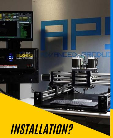
The start up process is very simple: The machine is already pre-assembled. Open the crate, place the SPYDER on a desk or stand, plug and start using.
